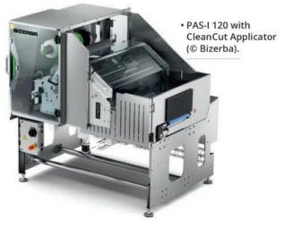
disposal costs. With its increased roll capacity and patented CleanCut\* technology that prevents adhesive residue on blades, downtime is minimised as the need for roll changes and blade cleaning are significantly extended.
